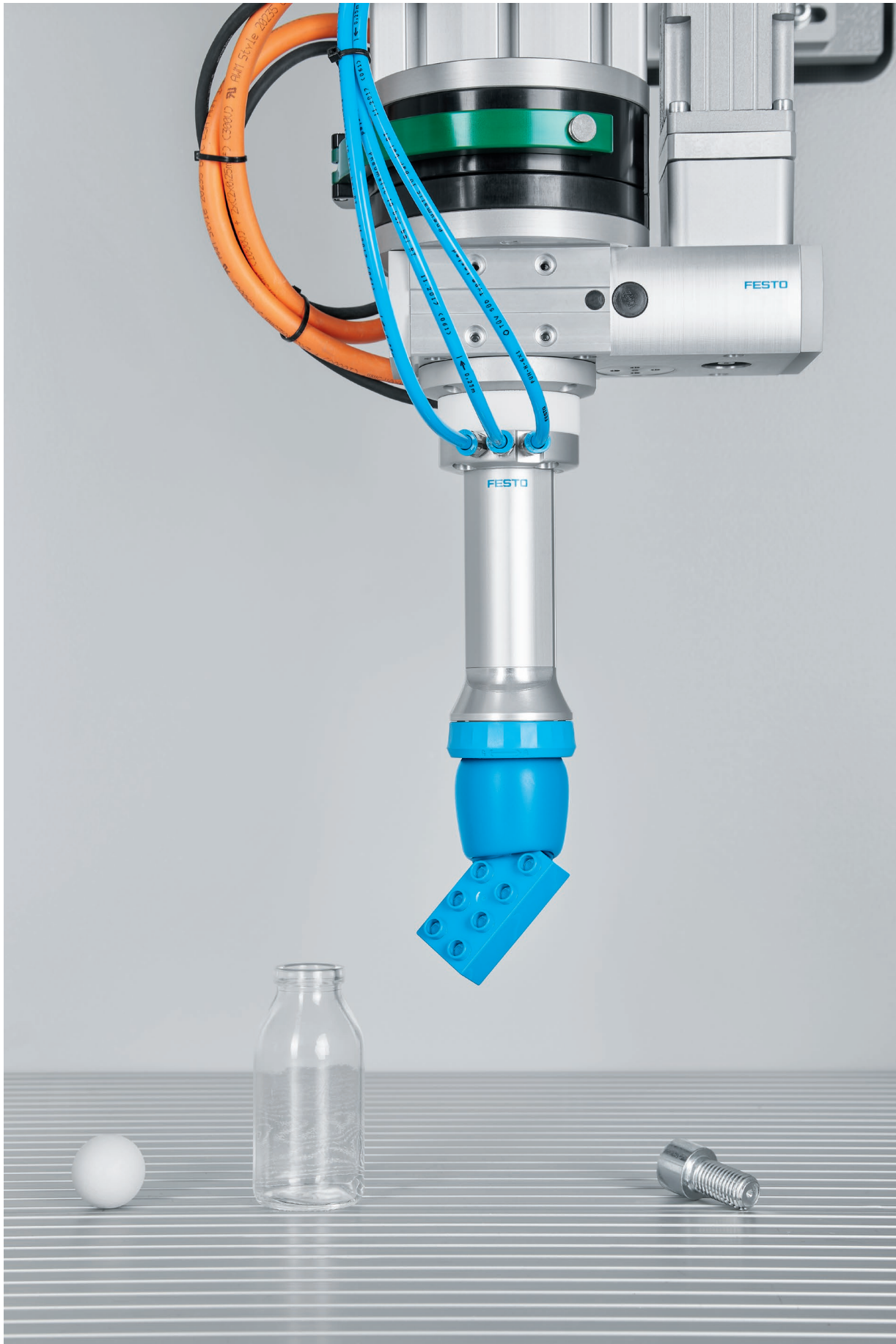
Learning from nature: the adaptive shape gripper is inspired by the chameleon's tongue. It can be used to grip objects with completely different contours and shapes.
