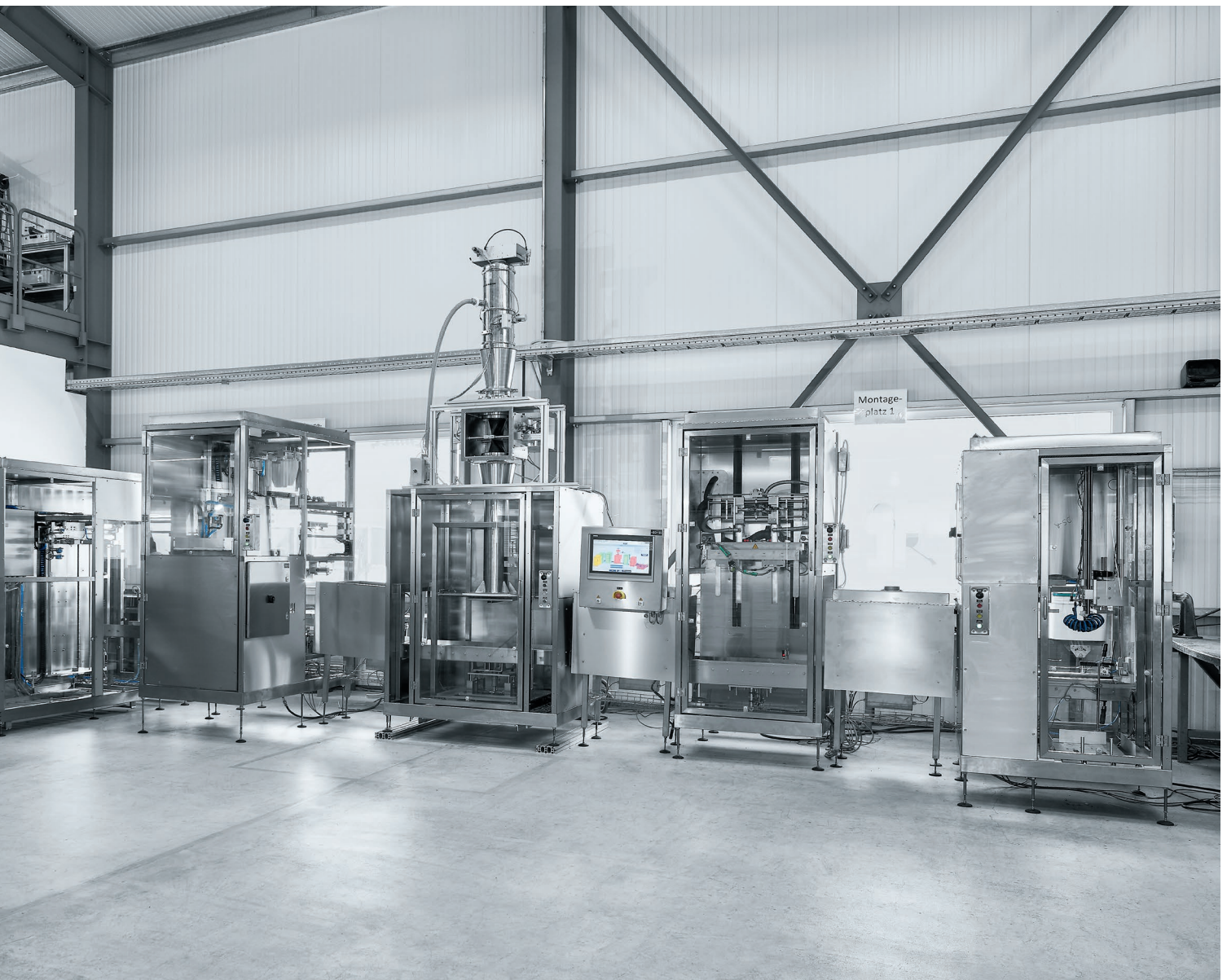
Greater productivity in fully automatic filling and hygienic packaging: the complete line developed by Burgener for pharmaceutical additives in powder form performs complex processes in a straightforward way. Components from Festo play an important role here.
